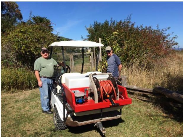
Thanks to the unique talents of one of our members, we now have the Chief's Golf Cart outfitted as a rapid attack vehicle. While small in stature (the cart, not the member) this vehicle can quickly move to help extinguish a fire in the incipient stages or contain the spread of the fire until our Tender and re-enforcements arrive.
